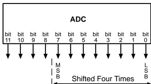
automatically be set to 1. Therefore, you should only use the multiply by 4 setting when your pixel readings with an 8 bit pixel format selected and with digital shift disabled are all less than 16.
