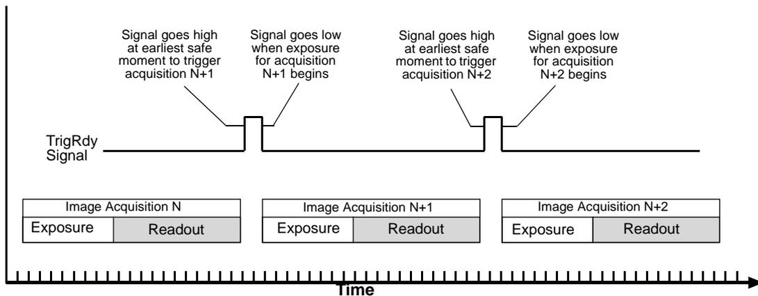
Fig. 52: Trigger Ready Signal
