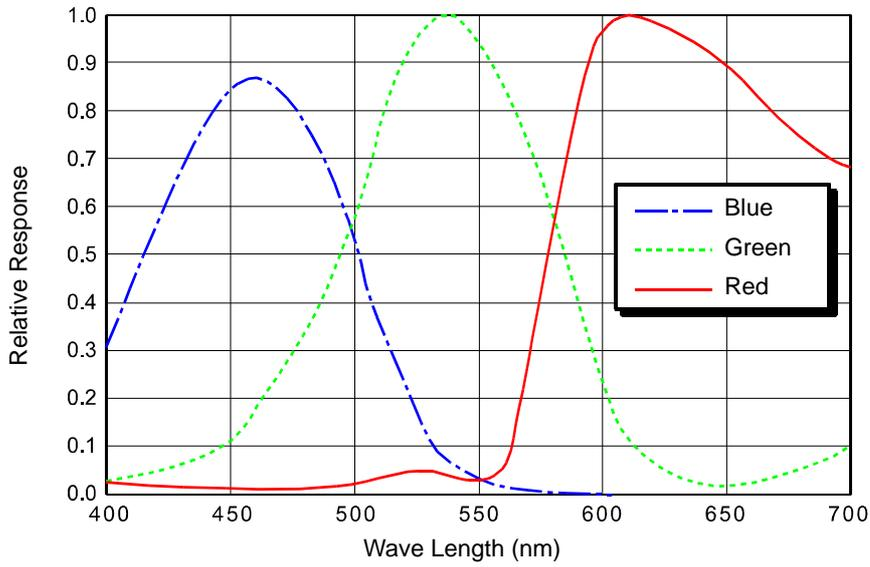
Fig. 16: scA1000-20gc and scA1000-30gc Spectral Response
