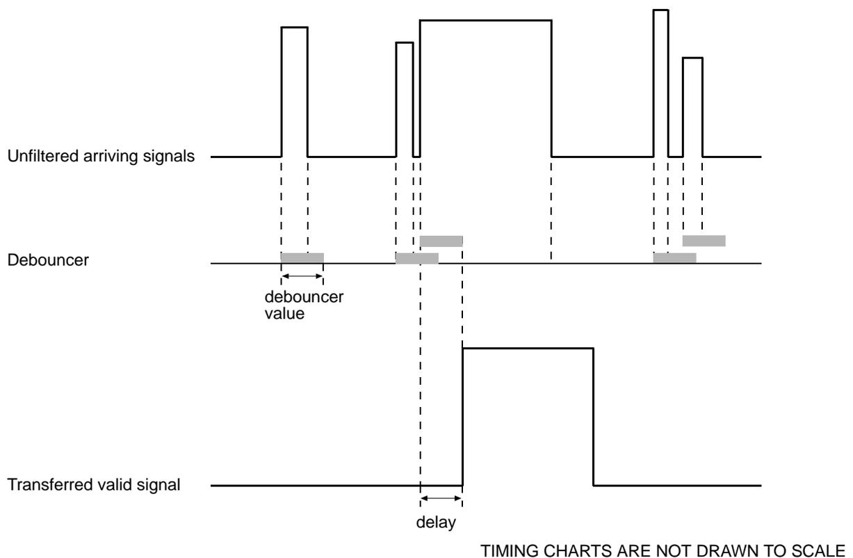
Fig. 71: Filtering of Input Signals by the Debouncer
