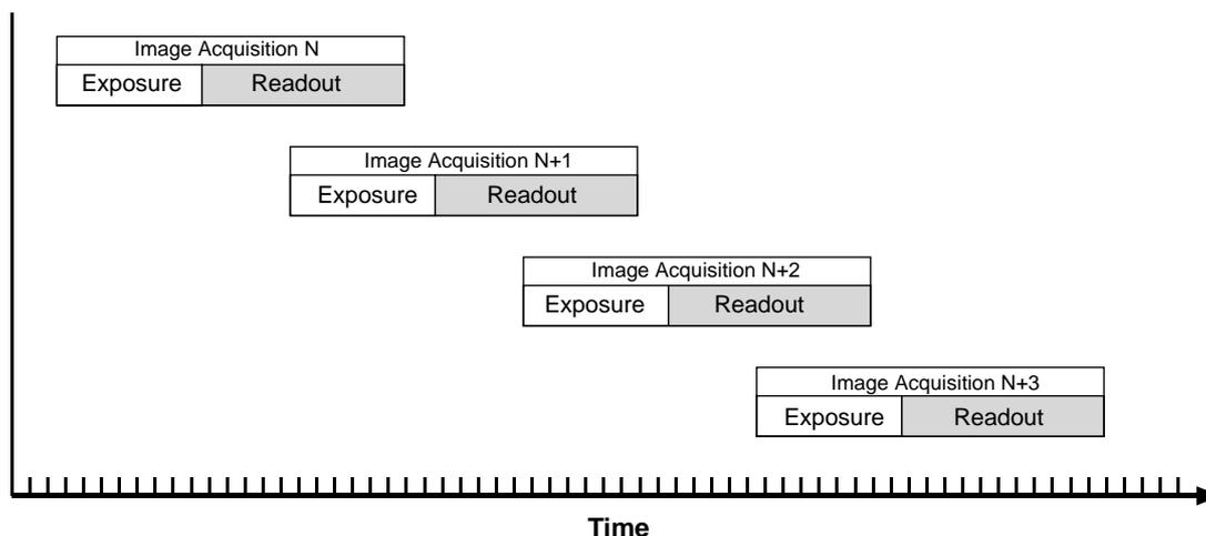
Fig. 49: Overlapped Exposure
