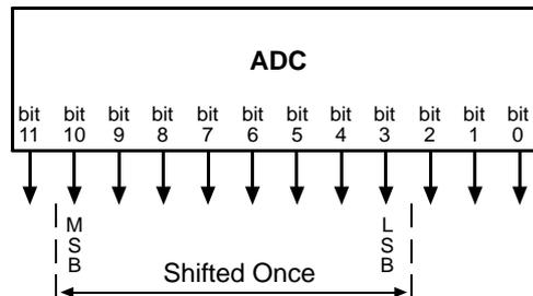
If the pixel values being output by the camera's sensor are high enough to set bit 11 to 1, we recommend not using shift by 1. If you do nonetheless, all bits output from the camera will automatically be set to 1. Therefore, you should only use the shift by 1 setting when your pixel readings with an 8 bit pixel format selected and with digital shift disabled are all less than 128.
