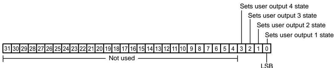
Fig. 56: User Output Value All Parameter Bits
