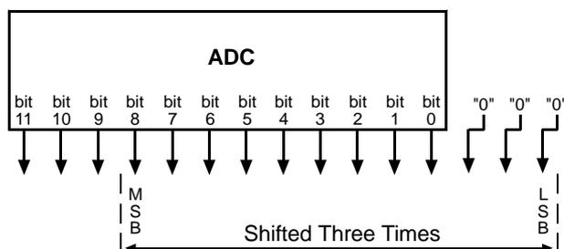
If the pixel values being output by the camera's sensor are high enough to set bit 9, bit 10, or bit 11 to 1, we recommend not using shift by 3. If you do nonetheless, all bits output from the camera will automatically be set to 1. Therefore, you should only use the shift by 3 setting when your pixel readings with a 12 bit pixel format selected and with digital shift disabled are all less than 512.
