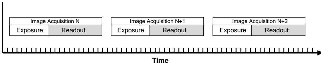
Fig. 48: Non-overlapped Exposure
