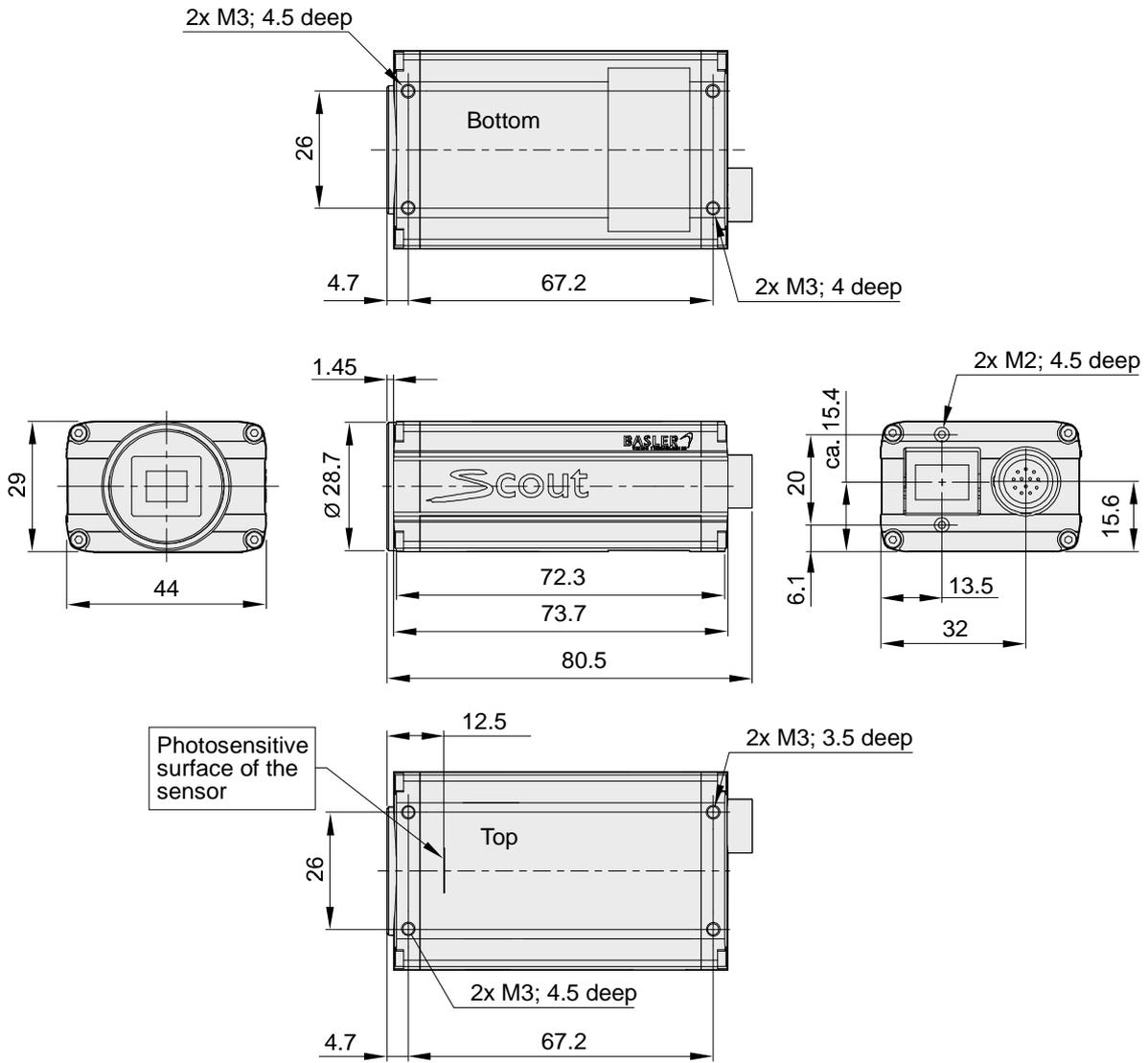
Fig. 22: Mechanical Dimensions (in mm) for Cameras with an Optional CS-mount Lens Adapter
