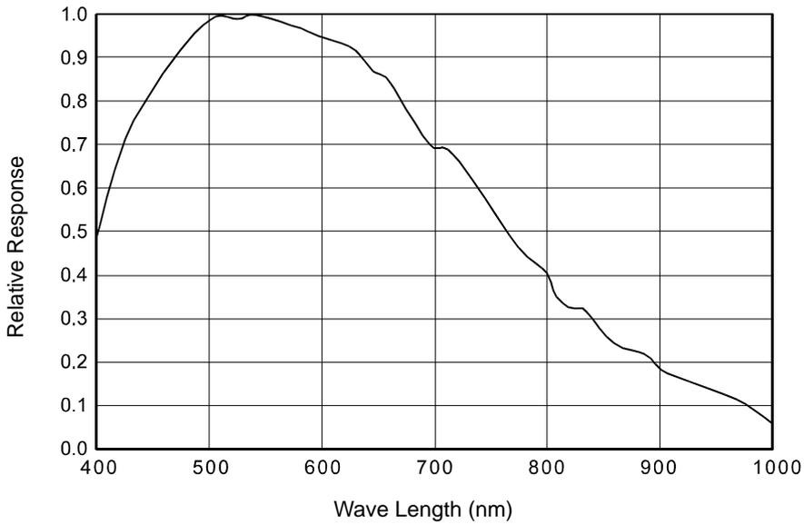
Fig. 9: scA1400-17gm and scA1400-30gm Spectral Response
