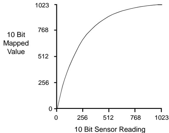
Fig. 68: Lookup Table with Values Mapped for Higher Camera Output at Low Sensor Readings
