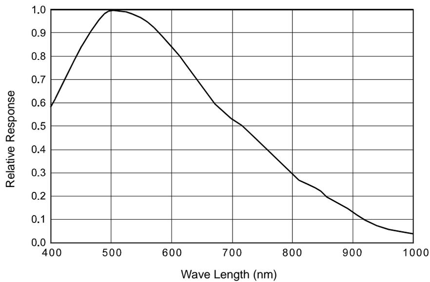
Fig. 5: scA780-54gm Spectral Response
