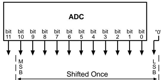
When the camera is set to shift by 1, the least significant bit output from the camera for each pixel value will be 0. This means that no odd gray values can be output and that the gray value scale will
