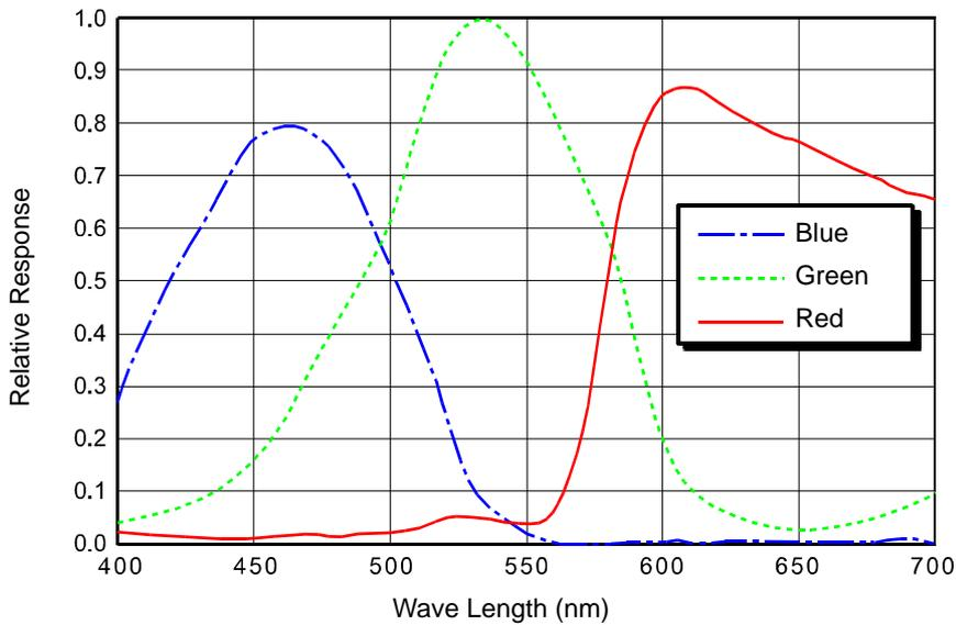
Fig. 11: scA640-70gc Spectral Response
