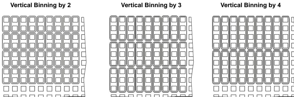
Fig. 61: Vertical Binning
