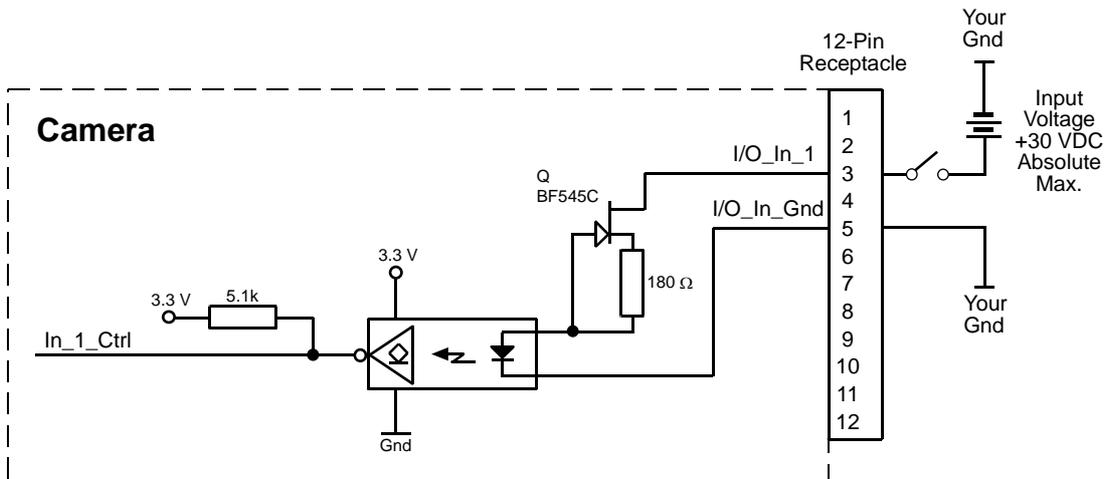
Fig. 39: Typical Input Circuit
