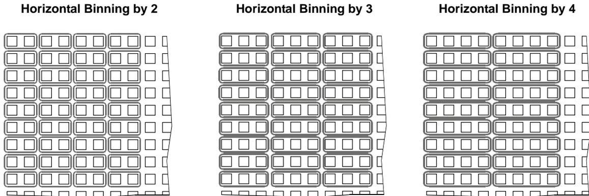
Fig. 62: Horizontal Binning
