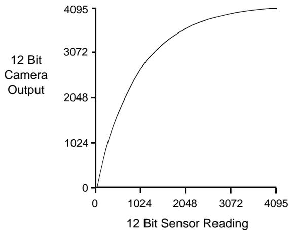
Fig. 66: Lookup Table with Values Mapped for Higher Camera Output at Low Sensor Readings
