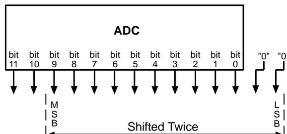
If the pixel values being output by the camera's sensor are high enough to set bit 10 or bit 11 to 1, we recommend not using shift by 2. If you do nonetheless, all bits output from the camera will automatically be set to 1. Therefore, you should only use the shift by 2 setting when your pixel readings with a 12 bit pixel format selected and with digital shift disabled are all less than 1024.
