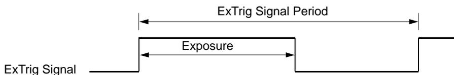
Fig. 46: Trigger Width Exposure with Rising Edge Triggering
