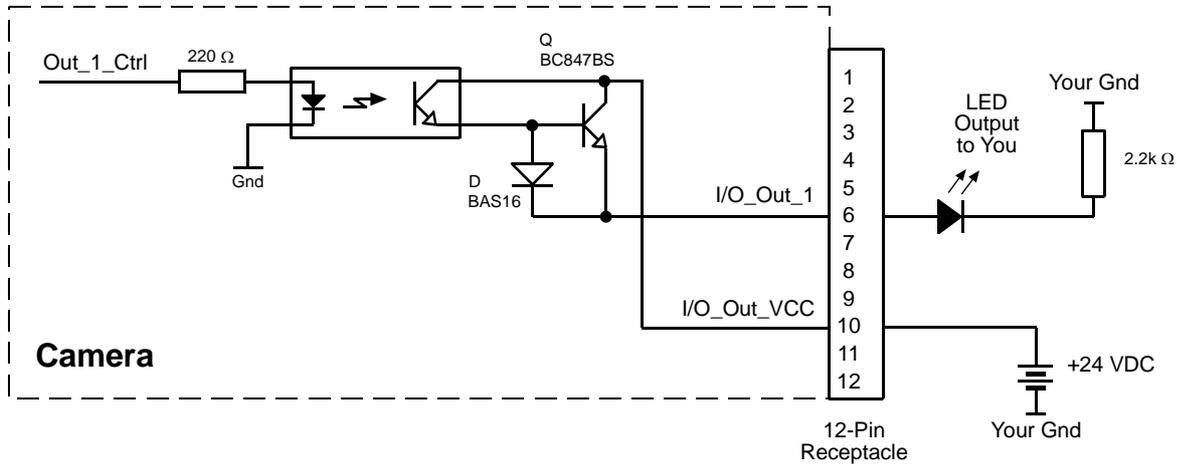
Fig. 41: Typical LED Output Signal at +24 VDC for the External Circuit (Example)
