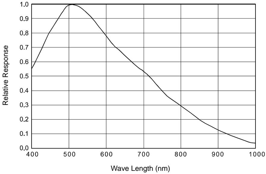
Fig. 6: scA1000-20gm and scA1000-30gm Spectral Response
