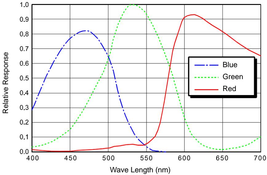
Fig. 15: scA780-54gc Spectral Response
