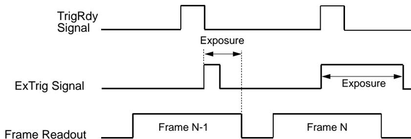
Fig. 47: Trigger Width Exposure Mode with Overlapped Exposure
