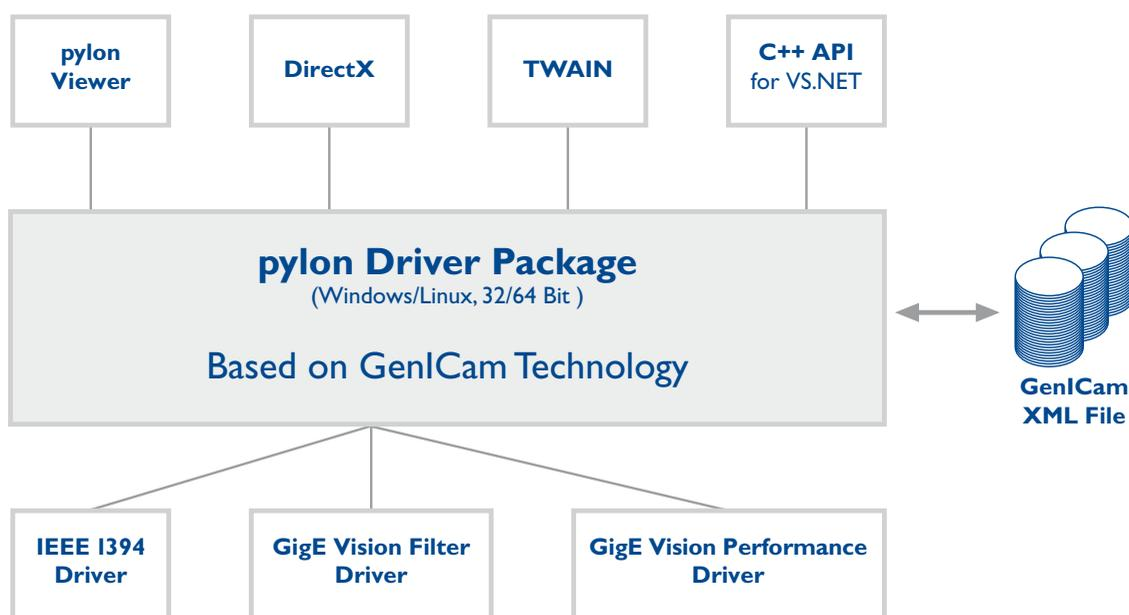
The internal architecture of the pylon driver package is based on GenICam Technology, which offers you easy access to the newest camera models and the latest features. Changes to an existing camera device in your application essentially become a plug-and-play process.
